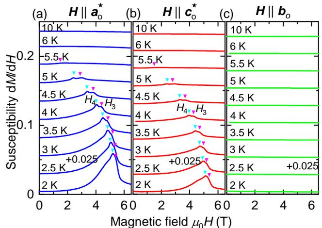
FIG. 6. (a) Susceptibility,  $dM/dH$ , calculated from the measured magnetization of orthorhombic CePdAl<sub>3</sub> for (a)  $\mathbf{H} \parallel \mathbf{a}_o^*$ , (b)  $\mathbf{H} \parallel \mathbf{c}_o^*$  and (c)  $\mathbf{H} \parallel \mathbf{b}_o$ . Data are shifted by 0.025 for clarity. Peaks correspond to field-induced transitions marked by arrows at  $H_3$  (pink) and  $H_4$  (sky blue). The peaks disappear above  $T_N$ .
